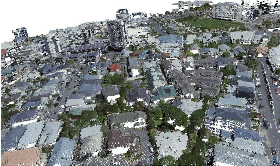
**Figure 3:** An example of a tile in the Wellington region, comprising 3D points and RGB colour values.
