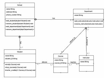
FIGURE 1 The UML Class diagram for School.
