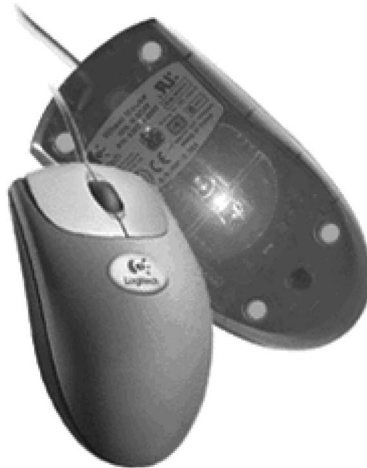
Figure 2. The Logitech iFeel mouse ( www.logitech.com ). The mouse looks and operates like an ordinary desktop mouse but contains a motor with an eccentric weight that generates a range of different types of simple vibrotactile feedback to the hand.
